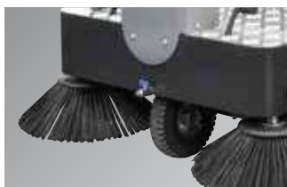
Front water system for dust reduction with 2lt rear tank
