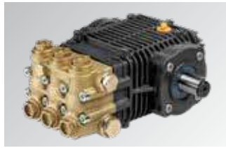
New CL 6.0 self-priming pump with three pistons in integral ceramic, tapered roller bearings, double oil viewer and brass head
