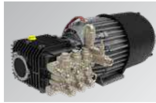
Professional motor pump with 4-pole motor (1400 rpm) and self-priming linear pump: the low rotation speed significantly extends the life of the components inside the motor pump, guaranteeing greater efficiency and silence
