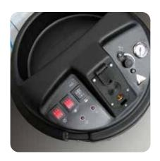
Simple and intuitive control panel, quick-coupling steam gun, main ON/OFF switch with lamp, boiler ON/OFF switch with lamp, water/detergent selector, steam flow rate regulator, steam ready indicator lamp, low water level indicator lamp with buzzer, steam pressure gauge. Steam gun with integrated steam/detergent function activation key and quick coupling of accessories.
